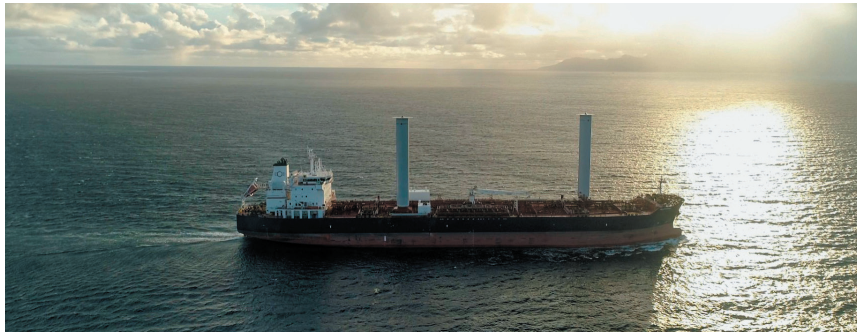
On the Alcyone , Norsepower's twin-mast rotors reduce greenhouse gas emissions by at least 10% on specific routes.
